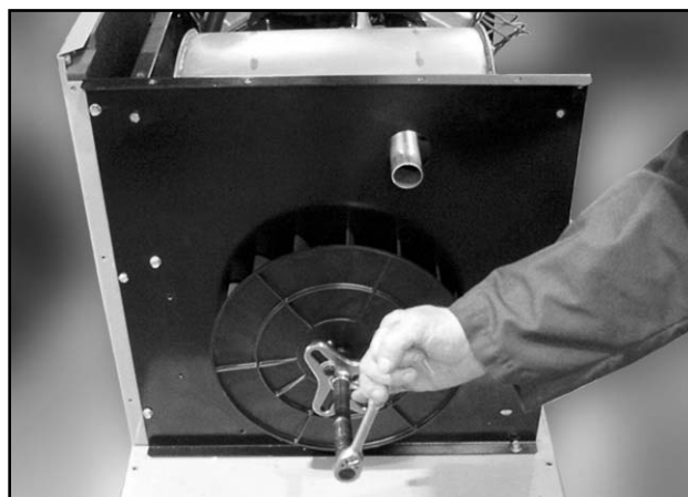
Figure 2. Using a Steering Wheel Puller to Remove Fan From Rotor
